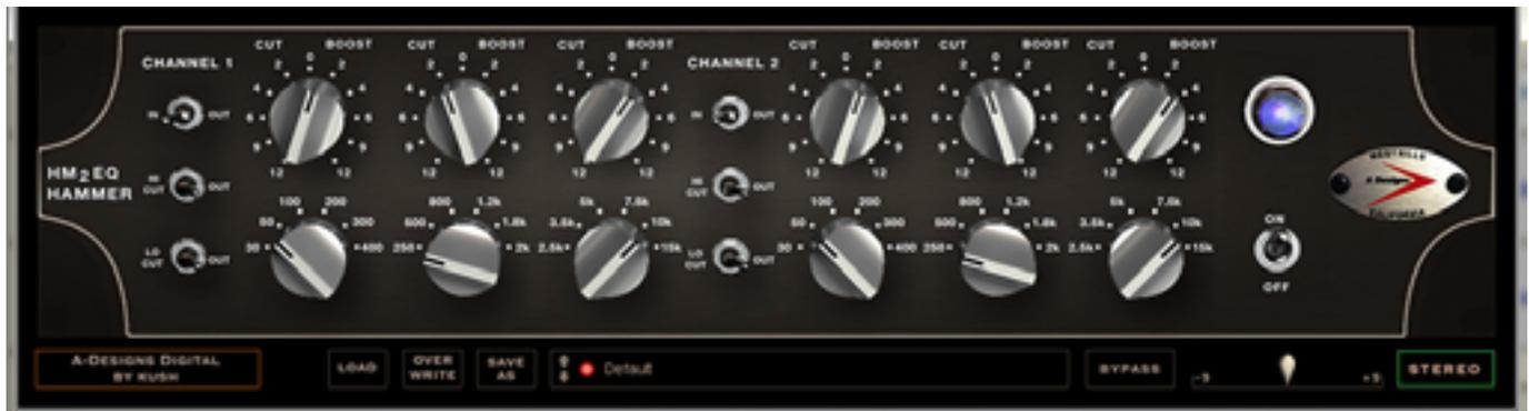
Channel 1      3 switches, for in/out,hi-cut/out, and lo-cut/out
