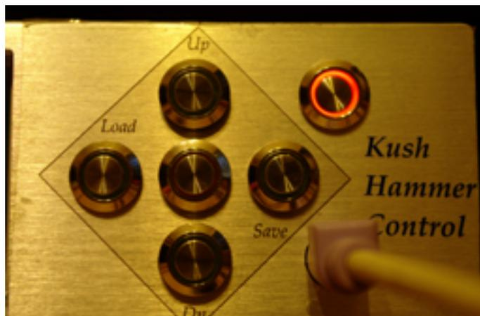
Press the load button, and the load button will flash, to show in load mode, and the up/select/down buttons in the middle will illuminate. Use the up/down buttons to scroll through presets, the values will update as you do so. To select a preset, use the centre button, and it will keep all the loaded values. To cancel, press the flashing load button again, which will put the values back to what they were before.
